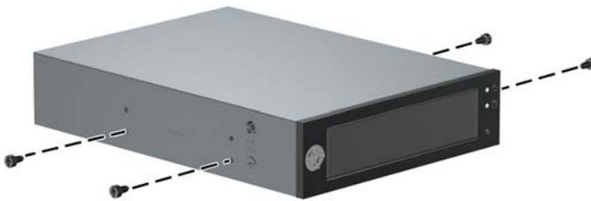
5. Position the guide screws on the drive into the J-slots in the drive bay. Then slide the drive toward the front of the computer until it locks into place.
