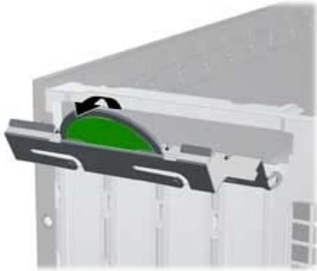
4. Remove the expansion card slot cover by pulling it up, out of the chassis.
