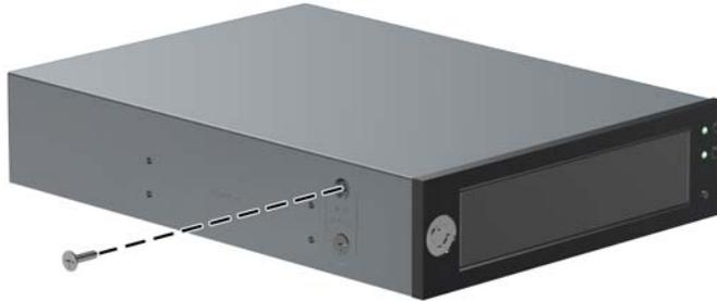
4. Install four (supplied) M3 x 5mm screws (black) in the lower four mounting holes of the DX115 case. (See [Locating extra guide screws on page 72](#) for screw locations.)
